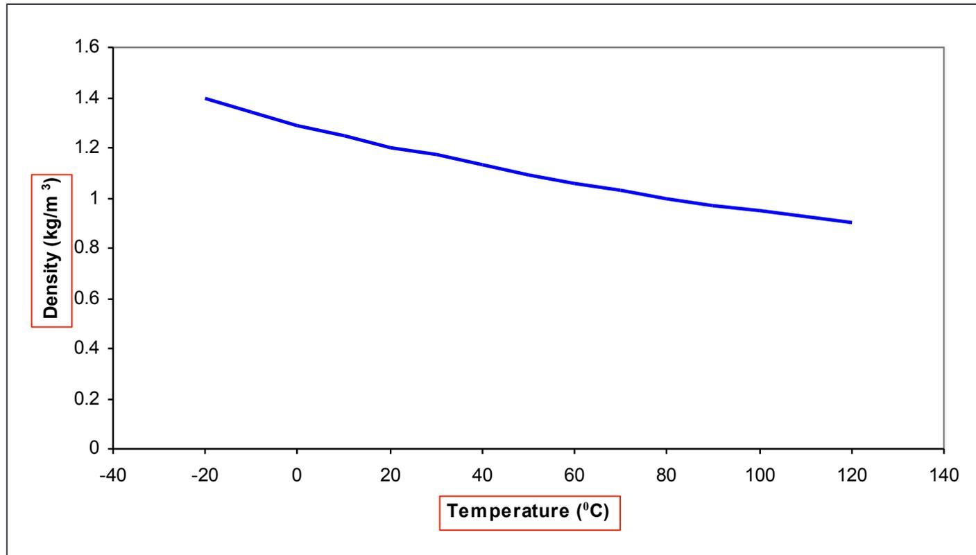
**Figure 3.** Relationship between density and temperature of air at standard atmospheric pressure. Source of data: Elger et al. (2001). *Engineering Fluid Mechanics*.
